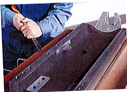
• Scraping of surface
