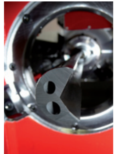
Deep drilling with single-lip deep drilling tools
