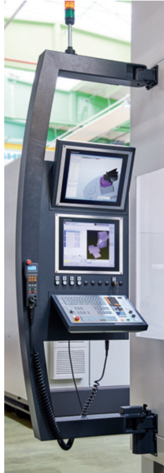
Control panel with control, Heidenhain TNC 640 (special network equipment for the workshop area, allows parallel working)
