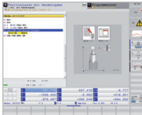
Easily and quickly applicable cycle for the kinematic measurement of the machine
