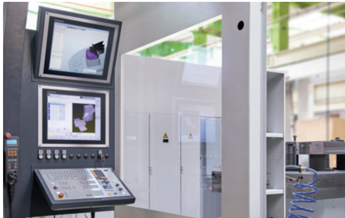
Control panel with control Heidenhain TNC 640 with additional monitor
