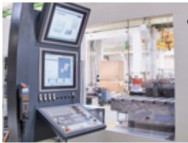
Swiveling control panel, inspection window towards the working area
