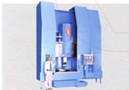
Completed full guarding
