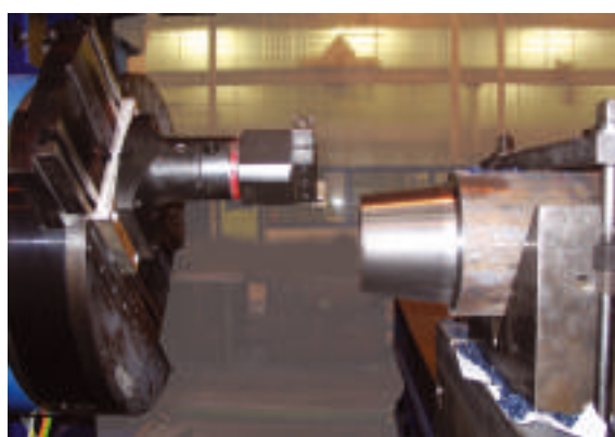
MILLING OF A FLANGE FOR PIPELINE
