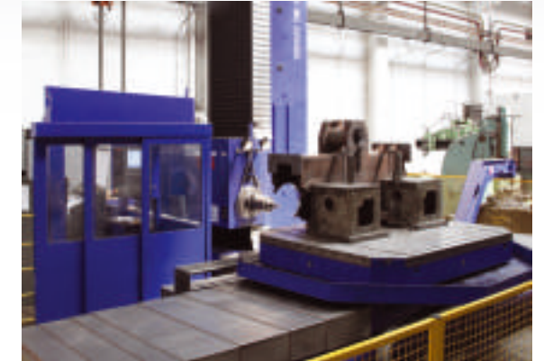
MILLING OF A HEAT EXCHANGER
