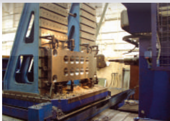
MILLING OF A HOLE INTRADOS
