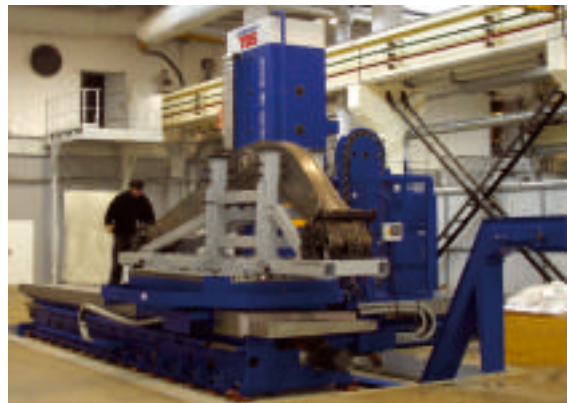
DOUBLE-SIDED MILLING OF A CRANE ARM
