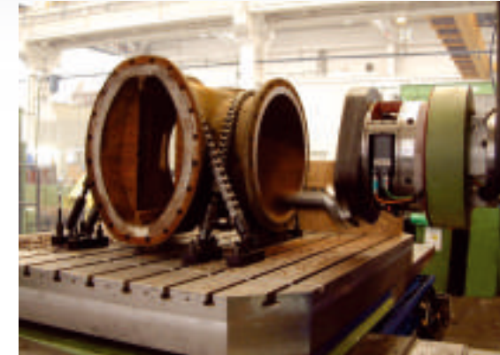
MILLING OF A VALVE FACE
