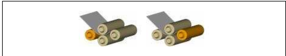
Figure 9.22 - Positioning steps for rolling
