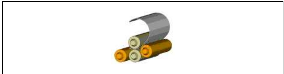
Figure 9.14 - Positioning steps for second rolling
