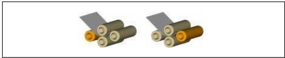
Figure 9.6 - Positioning steps for rolling
