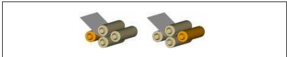
Figure 9.10 - Positioning steps for rolling
