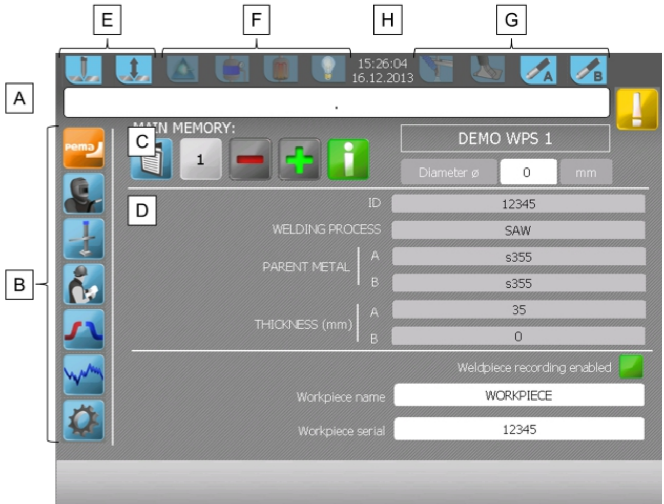
Figure 11 OP1 touch panel structure
