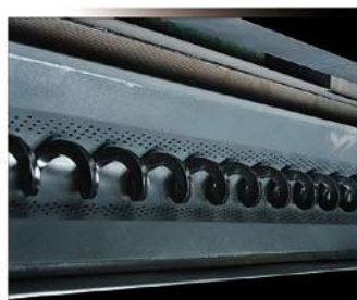
Automatic chip removal (Screw type chip conveyor)
