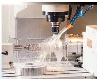
High pressure coolant (P:3.5 kg/cm 2 , Q:100 l/min)
