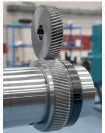
the spindle powertrain uses hardened and ground gears
