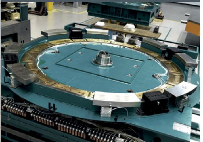
hydrostatic thrust bearing and hydrostatic pads
