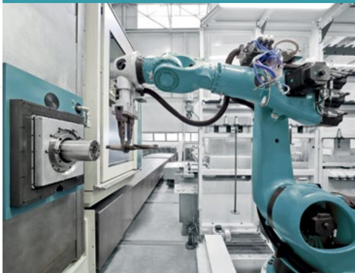
rack type tool magazines, floor mounted and served by robot, with capacity up to 1000 tools
