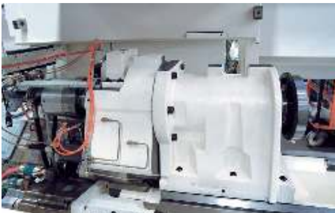
To avoid influences caused by heat transfer, the headstock and gearbox are thermally separated. The bearings of the main spindle are manufactured to the same high standards as those used on VDF Boehringer CNC turning machines
