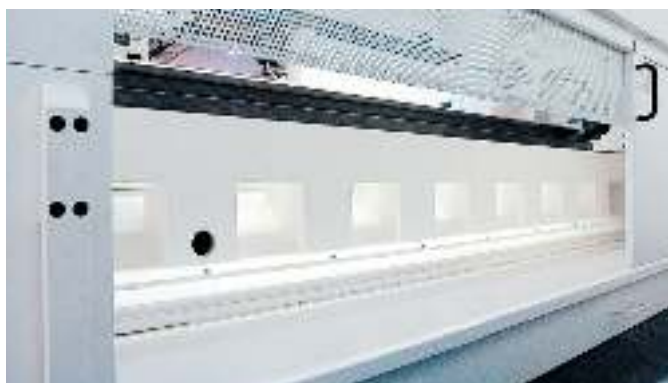
Large chip chutes in the machine bed provide efficient chip disposal. The chips can easily be removed from the chip pan through the sliding doors on the back side
