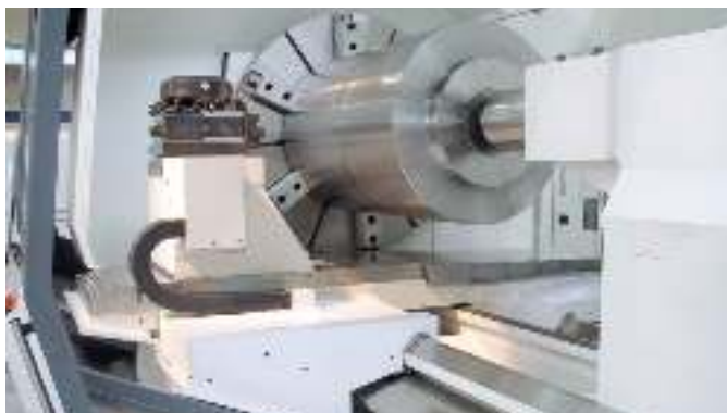
Working area with 4-position universal turret
