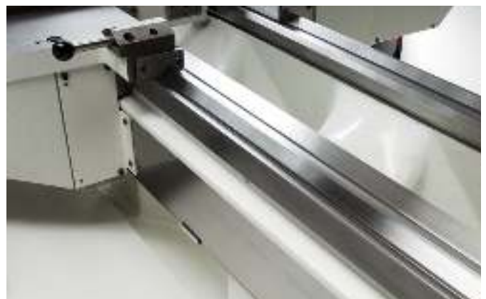
The guideways for the carriage (double vee) and the tailstock (vee and flat guideway) are a well proven combination. Large slideway surface areas with low surface pressure ensures high guiding efficiency with high long-term precision and repetitive accuracy
