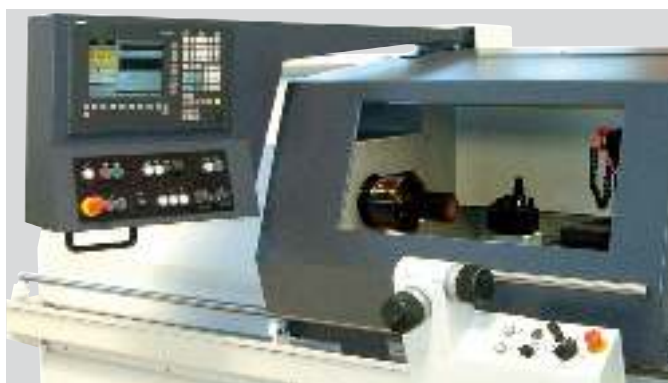
Pivoting control panel. Non-traveling chip protection door
