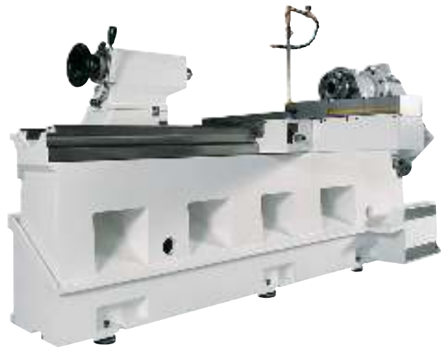
The basis for high turning efficiency and lasting accuracy is the heavy, rigid box-type bed with large chip chutes to the rear
