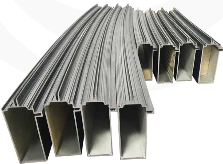
Curved 250 x 100 frame sections. zero distortion using Inductaflex Bio-fler
